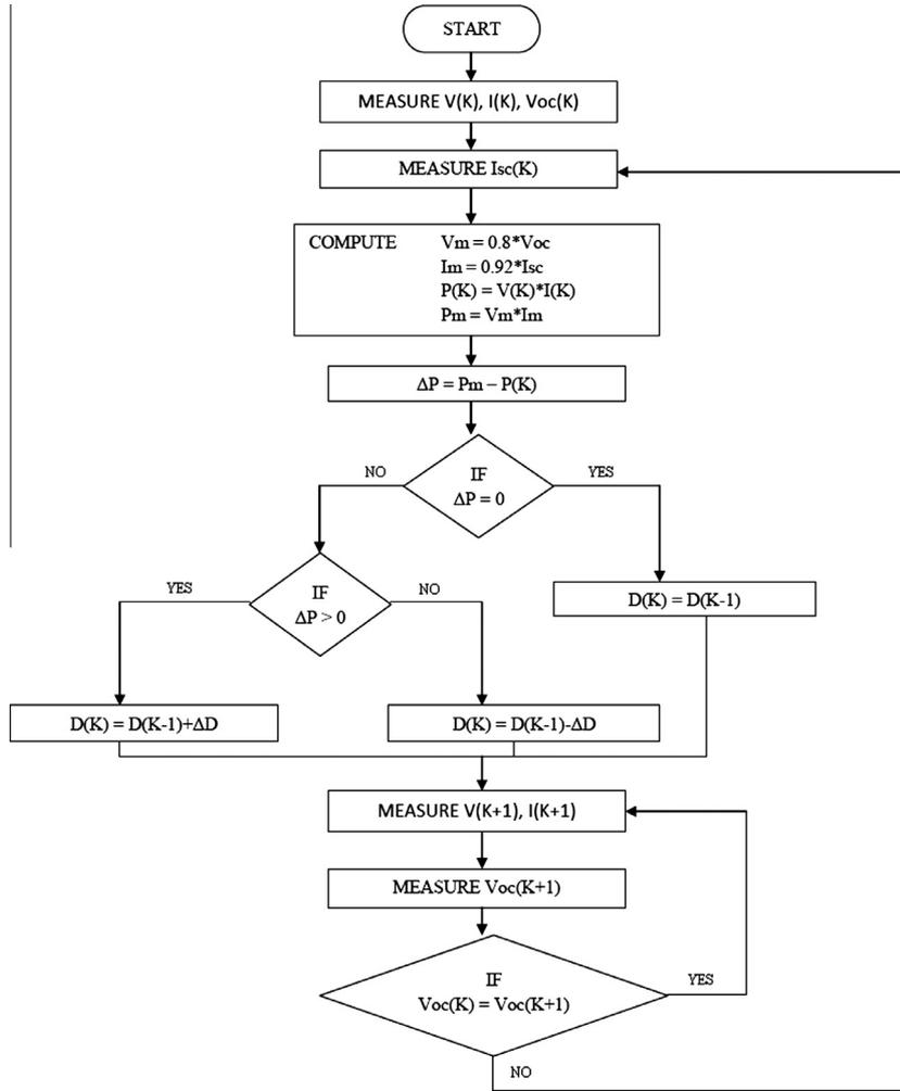
Fig. 1. Flow chart of proposed MPPT algorithm.
