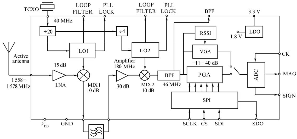
Fig. 1 Block diagram of the GPS receiver
