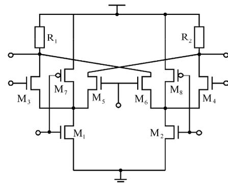
Fig. 3 Schematic of RF mixer
