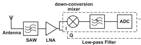
Fig. 1. Direct I/Q conversion receiver.
