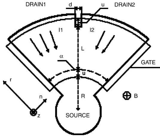
Fig. 1. Layout of sector MAGFET with geometrical parameters.
