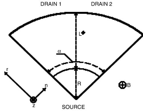
Fig. 2. Modified channel region of the sector MAGFET (the transformed drain distance is zero).
