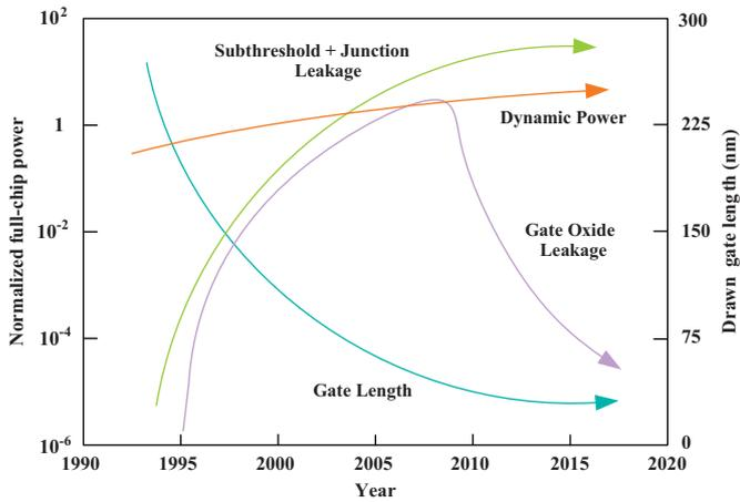
Fig. 1. Total chip dynamic and static power dissipation trends based on the International Technology Roadmap for Semiconductors [3]. Gate oxide leakage is under control by using high-k dielectrics [30,19].
