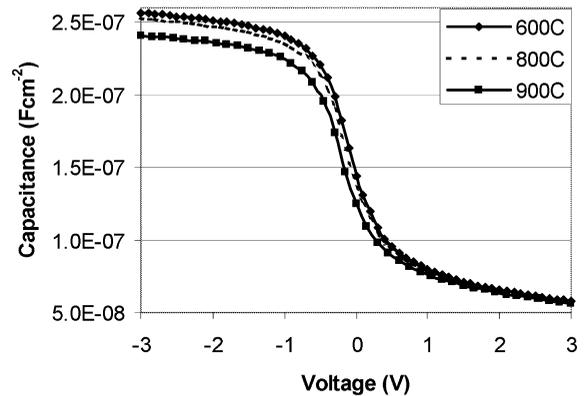
Fig. 2. High frequency CV characteristics on the Ir/SiO<sub>2</sub>/Si capacitors with 15-nm dielectric thickness annealed in N<sub>2</sub> to 600, 800 and 900 °C followed by FGA at 420 °C for 20 min. The flat band voltage shift corresponds to the change in effective oxide charges.
