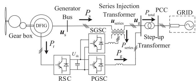
Fig. 1. Configuration of DFIG system with SGSC.
