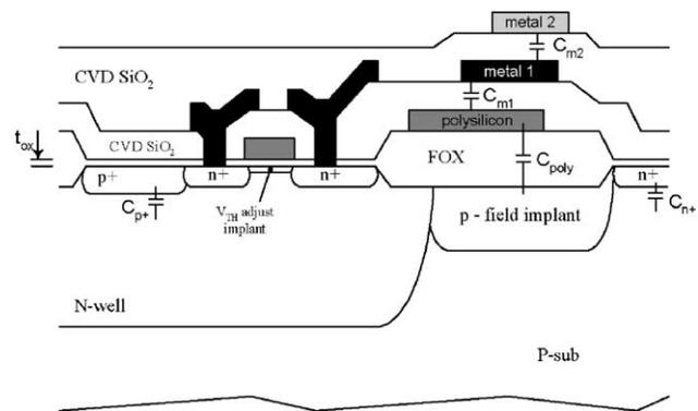
Fig. 1. Cross-section for an N-well CMOS typical process.
