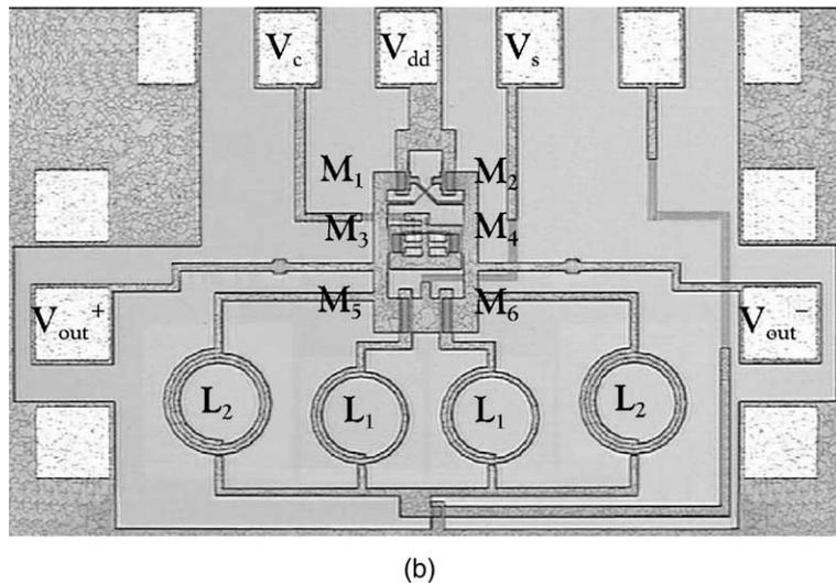
Fig. 1. Circuit schematics of a monolithic CMOS dual-band VCO (a), die photograph of the dual-band VCO fabricated by 0.18  $\mu\text{m}$  technologies (b).
