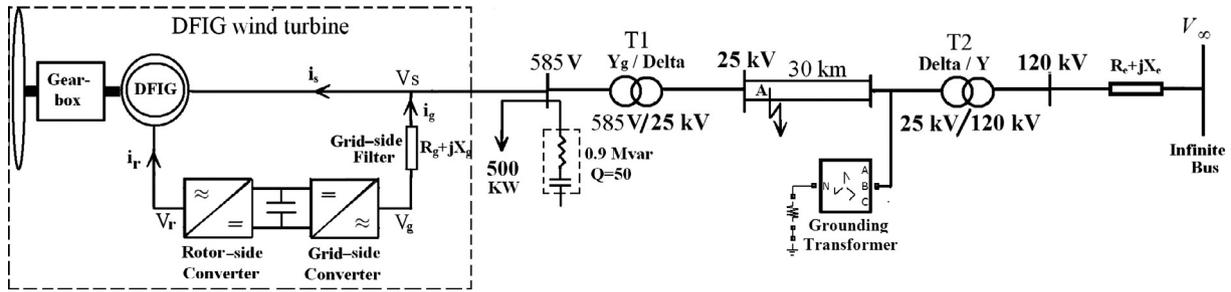
Fig. 1. Schematic diagram of the study system.
