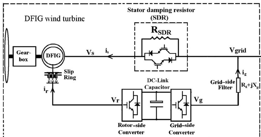
Fig. 2. Schematic diagram of SDR.
