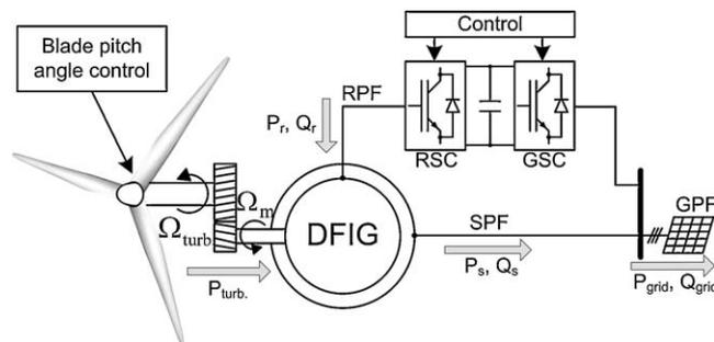
Fig. 1. DFIG wind turbine system components.
