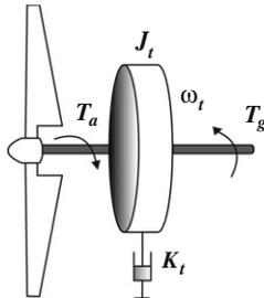
Fig. 1. One mass wind turbine model dynamics.
