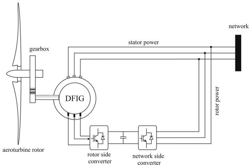
Fig. 2. Configuration scheme of a DFIG-based wind turbine.
