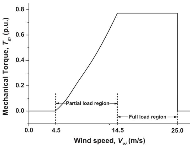
Fig. 3. Operating regions of the DFIG wind turbine at the turbine rotor speed of 1 p.u.
