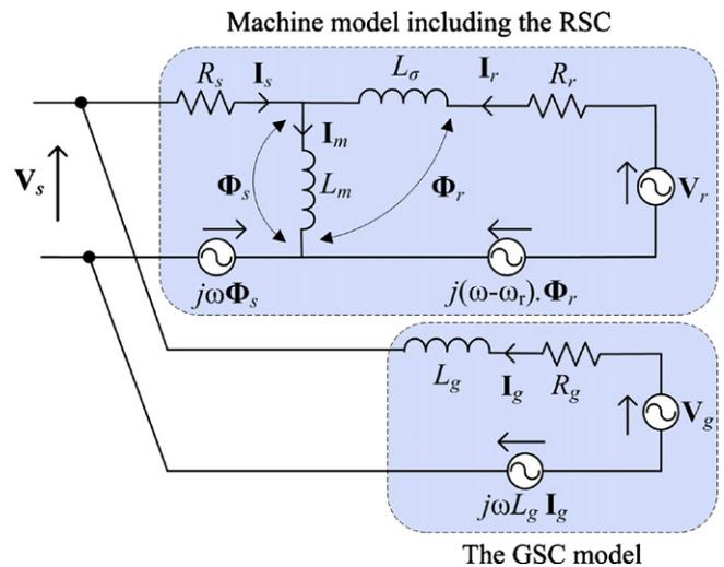
Fig. 2. Conventional  $\Gamma$ -form equivalent circuit of DFIG.
