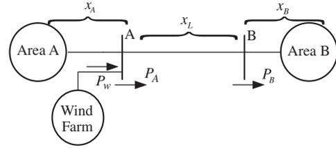
Fig. 1. Two-area power system integrated with a wind farm.
