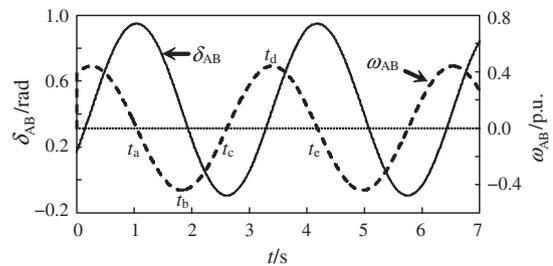
Fig. 2. Oscillation characteristics of  $\delta_{AB}$  and  $\omega_{AB}$  in a zero damping power system.
