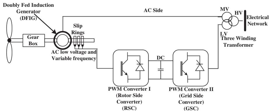
Fig. 1. Schematic of DFIG integrated with electrical grid.
