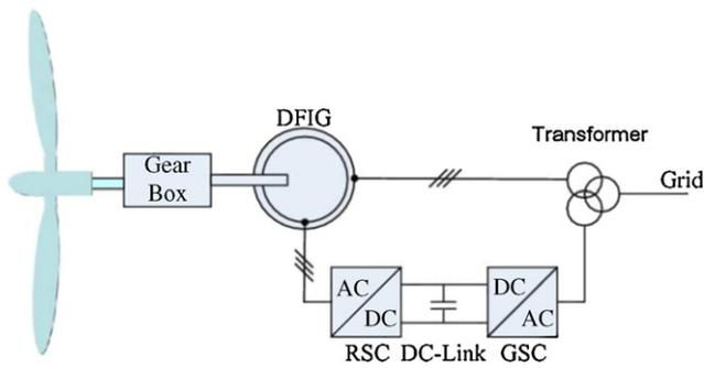
Fig. 1. Schematic diagram of a DFIG-based wind generation system.
