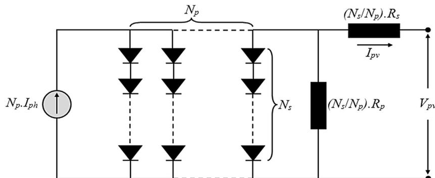
Fig. 1 – Equivalent circuit of the photovoltaic panel.
