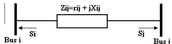
Fig. 2. TCSC injection model.
