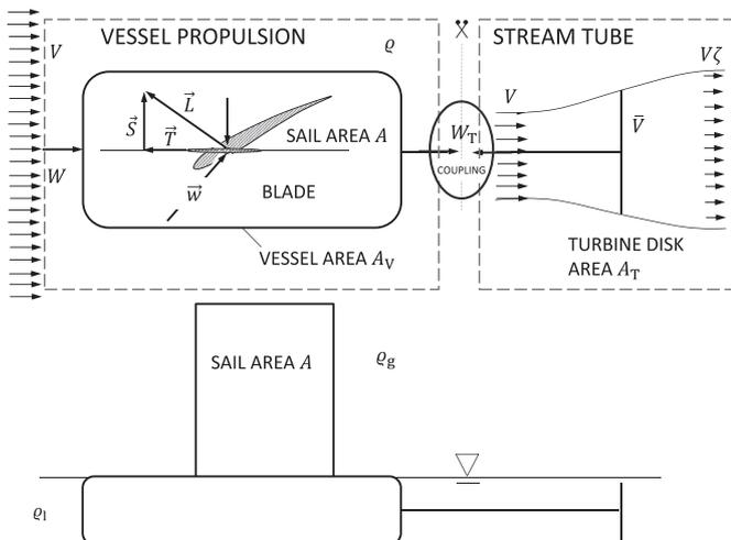
Fig. 1. Free-body representation of the energy ship.
