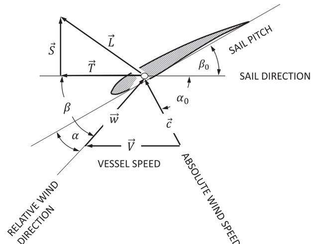
Fig. 2. Wind speed and forces on a sail section.
