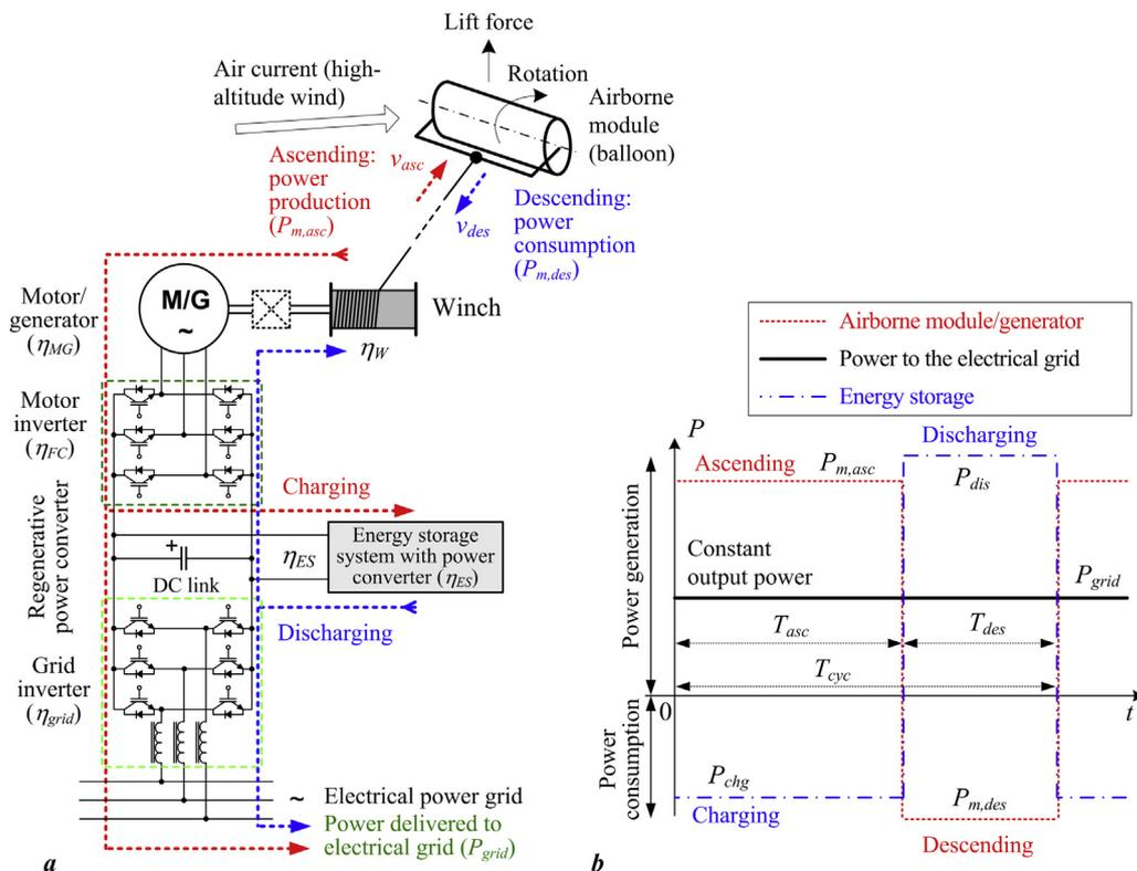
Fig. 1. Simplified representation of HAWC system (a) and illustration of its power cycle (b).
