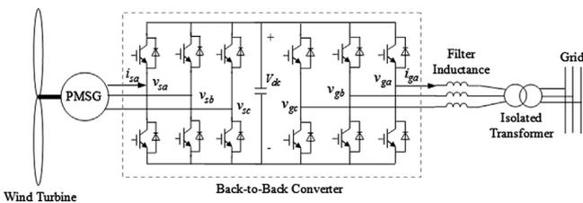
Fig. 1. Configuration of DDWECS.
