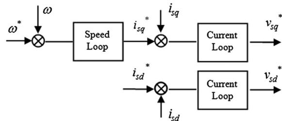
Fig. 2. Vector control structure for machine-side converter.
