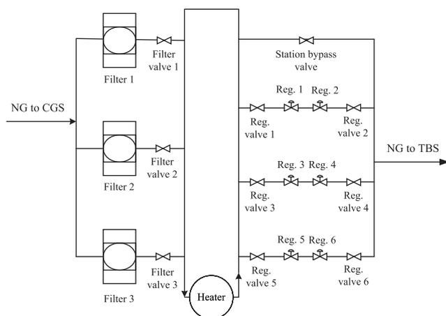
Fig. 1. Flow diagram of NG city gate station.
