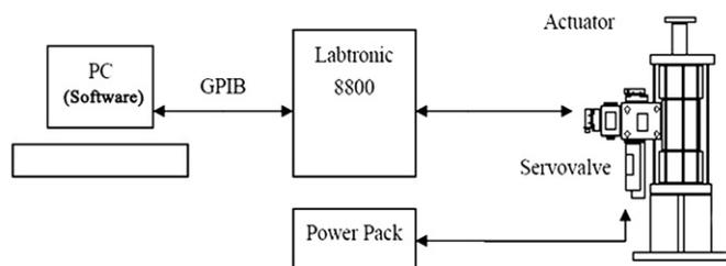
Fig. 1 – The road simulation test bench.
