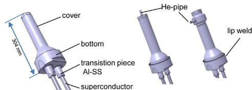
Fig. 1. Types of joint housings.
