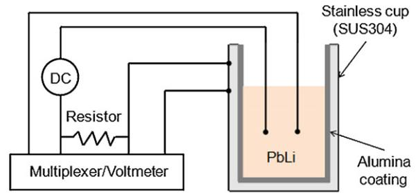
Fig. 1. Electrical insulation test.
