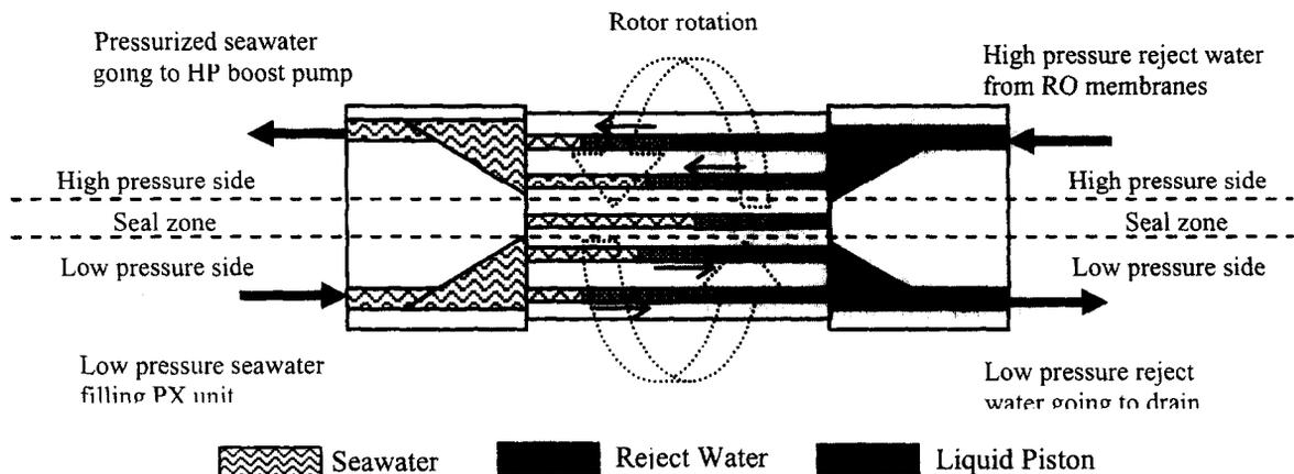
Fig. 1. Pressure exchanger flow path.
