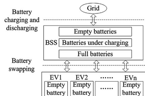
Fig. 1. The structure of EVs' power supply through BSS.
