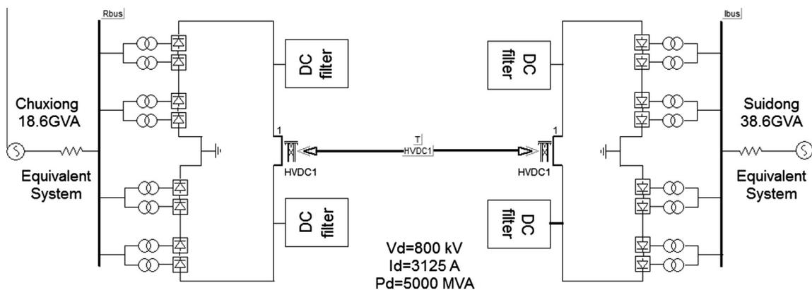
Fig. 1. HVDC structure diagram and equivalent system.
