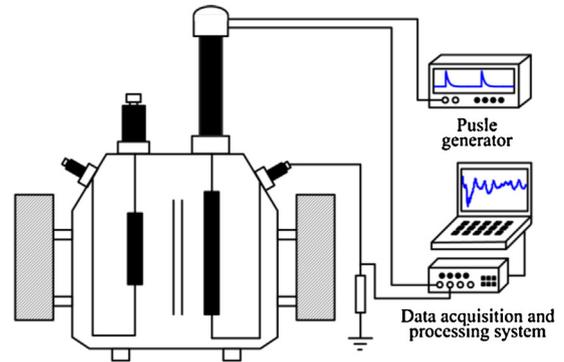
Fig. 1. Experiment setup of the LVI method.
