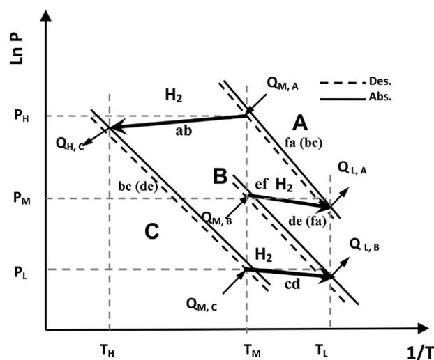
Fig. 1 – Operation of a DS-MHHT on van't Hoff plot.
