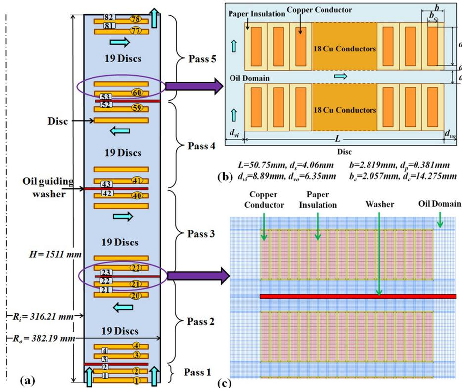
Fig. 1. (a) Geometry of the winding; (b) close up view of the different components of the winding; and (c) computational mesh for different fluid and solid domains. Numbering is presented in (a) for the discs as well as horizontal/radial channels.
