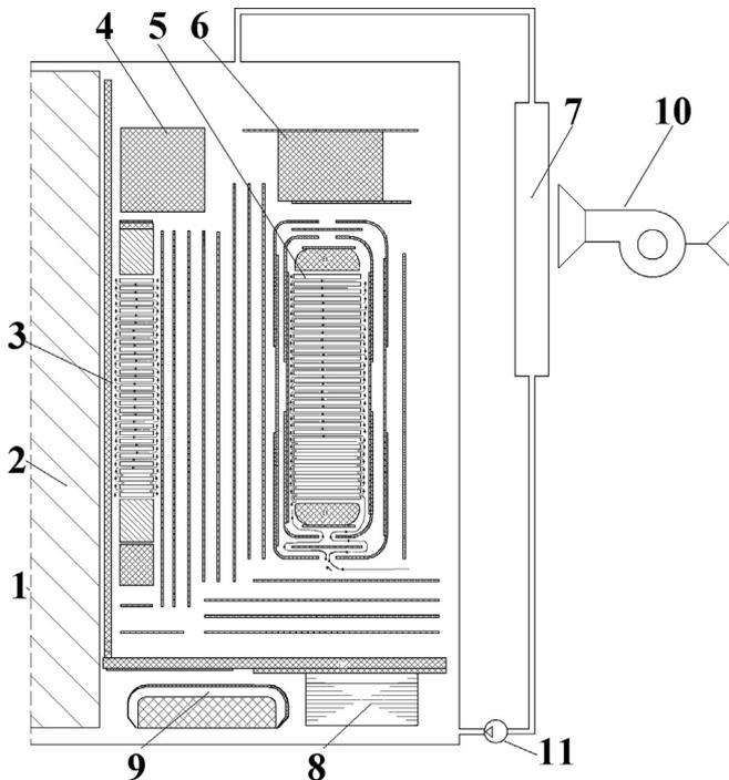
**Fig. 1.** The scheme of 210 MVA power transformer: 1 – axis of symmetry; 2 – transformer core; 3 – lower voltage winding (LV); 4 – pressing ring above LV winding; 5 – high-voltage winding (HV); 6 – pressing ring above HV winding; 7 – radiator of external cooling subsystem; 8 – shunt under HV winding; 9 – shunt under LV winding; 10 – fan; 11 – oil pump.
