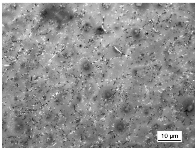
Fig. 2. Microscopic picture of the dispersed-CNF mixture.
