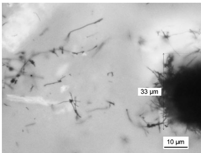
Fig. 1. Microscopic picture of the aggregated-CNF mixture; the measured diameter of the CNF aggregate is marked.
