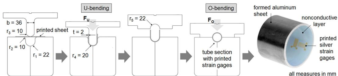
Fig. 1. Forming process for the manufacturing of printed tube sections with strain gages on the inner or outer surface [17, modified].
