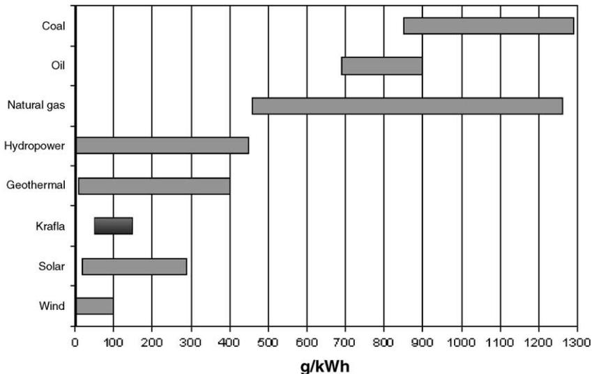
Fig. 1. Greenhouse gas emissions from various types of energy sources during generation of electricity. The emissions are expressed as CO<sub>2</sub> equivalents (Hunt, 2001; Armannsson et al., 2001). Krafla has one of the highest CO<sub>2</sub> emissions of the Icelandic geothermal fields.
