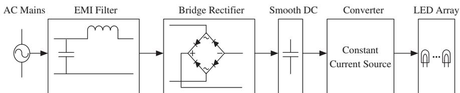
Fig. 1. Basic block diagram of LED lamp internal ballast circuit.
