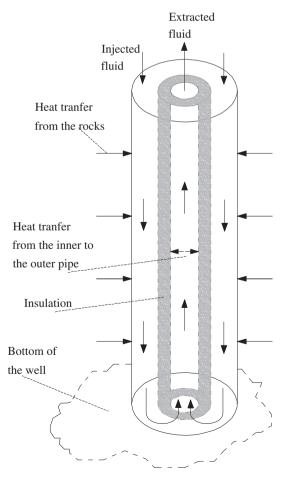
Fig. 1. Schematic representation of heat exchange in the single well.
