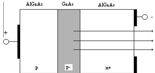
Fig. 4. Heterojunction structure.
