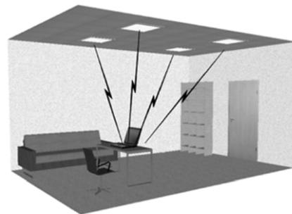
**Fig. 1** Visible light communication system using LED
