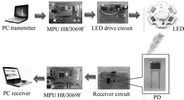
Fig. 2 Block diagram of visible light communication
