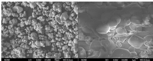
Fig. 2. SEM images of  $\text{Zn}_2\text{V}_2\text{O}_7$  sintered at a  $600^\circ\text{C}$ .
