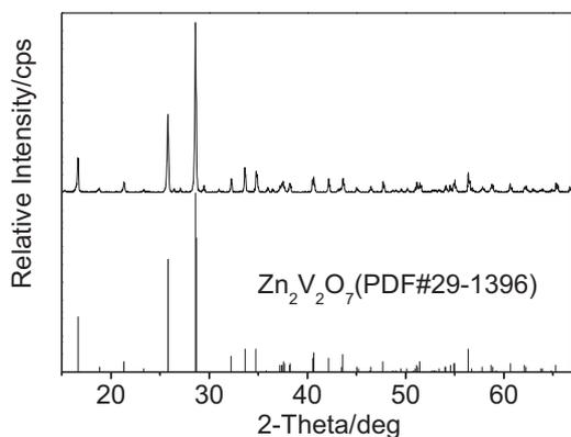
Fig. 1. XRD patterns of  $\text{Zn}_2\text{V}_2\text{O}_7$  prepared at  $600^\circ\text{C}$ .
