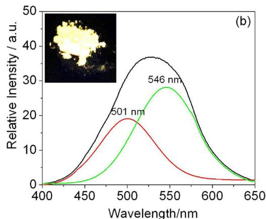
Fig. 3. Photoluminescence spectra of  $\text{Zn}_2\text{V}_2\text{O}_7$ : (a) excitation spectra ( $\lambda_{em} = 531\text{ nm}$ ); (b) emission spectra ( $\lambda_{ex} = 340\text{ nm}$ ). Inset: the photograph of  $\text{Zn}_2\text{V}_2\text{O}_7$  under ultraviolet light irradiation.
