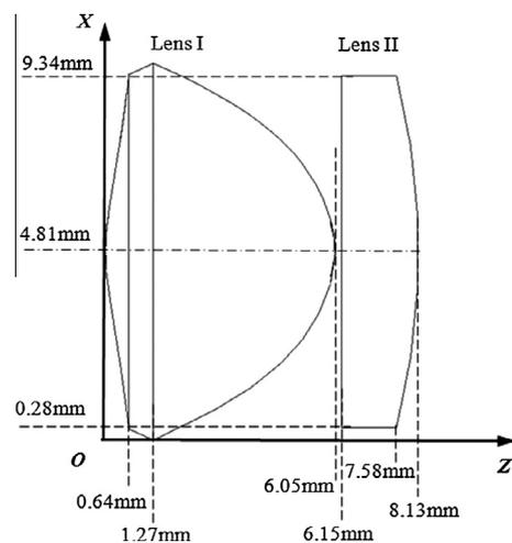
**Fig. 2.** Cross-section of the two illumination lenses.
