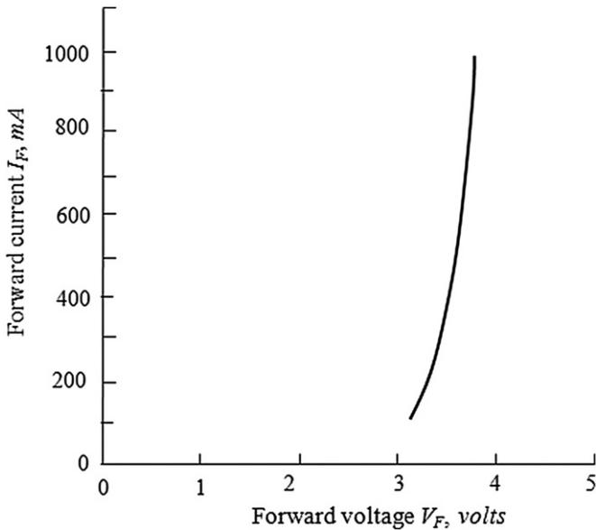
Fig. 1. I–V curve of an LED.
