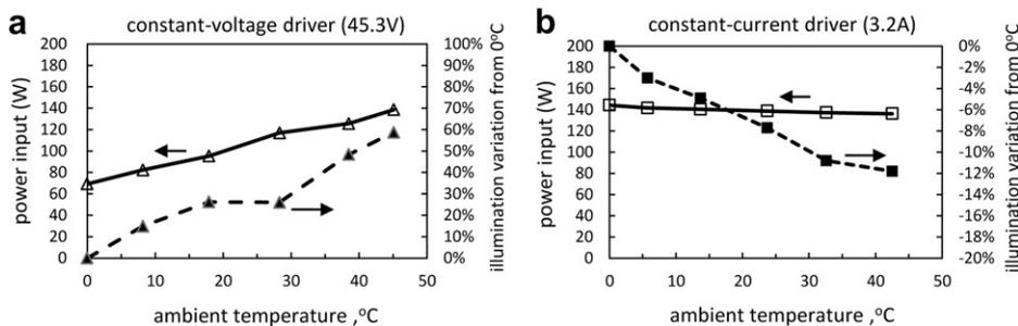
Fig. 2. Variation of LED illumination with temperature for different driver.
