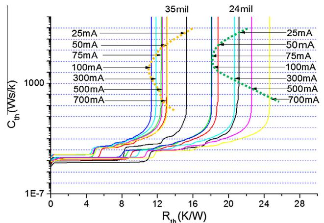
Fig. 2. Cumulative structure function for the 24 and 35 mil LEDs using variable input currents.
