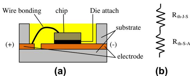
Fig. 1. LED schematic structure and the equivalent thermal circuit. (a) Package structure and (b) equivalent thermal resistance.
