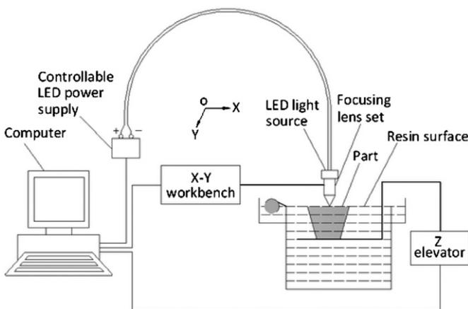
Fig. 2. Schematic diagram of LED-SL.
