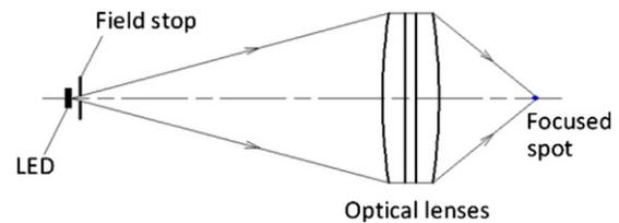
Fig. 4. Focus of the UV-LED light.
