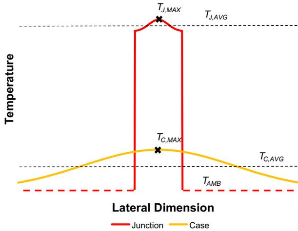
Fig. 1. Illustration: Junction and case temperature profiles for a one-chip LED package. Characteristic temperatures are indicated by crosses and dashed lines. The inhomogeneity of the profiles is clearly observable.
