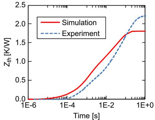
Fig. 3. Comparison of thermal transient data obtained from experiment and simulation.
