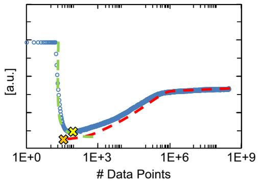
Fig. 4. Illustration: Parasitic electrical transient (green line) superimposed on the actual thermal signal (red line) results in the real measurement signal (blue line) and artifacts in the  $R_{th}$  extraction. (For interpretation of the references to color in this figure legend, the reader is referred to the web version of this article.)
