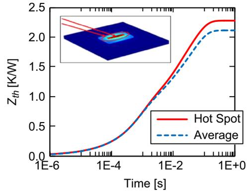
Fig. 2. Simulated thermal impedance graphs extracted at junction hot-spot (solid line) and averaged over all five LED chips (dashed line).
