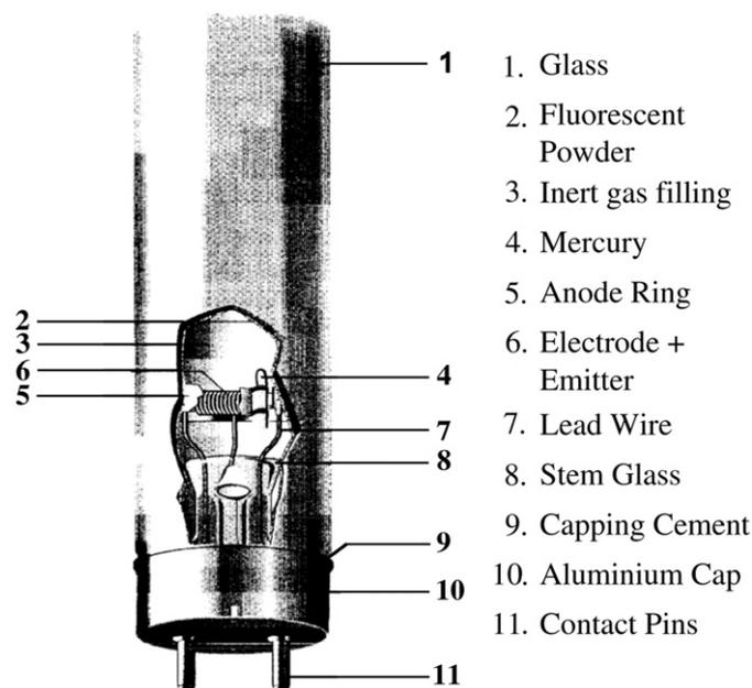
Fig. 1. The components of a fluorescent lamp [11].
