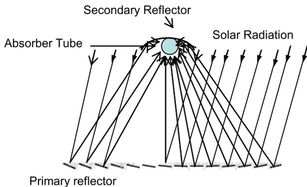
**Fig. 1.** Cross sectional view of the schematic diagram of a linear Fresnel collector. Laser aligned primary mirrors reflect the incoming light onto the absorber tube. Any leaked radiation strikes the secondary reflector and is reflected back to the tube.
