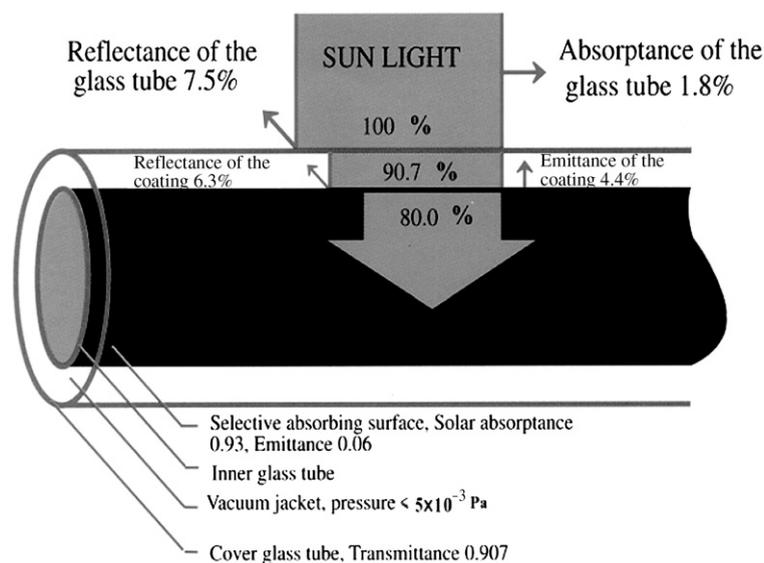
Fig. 1. A typical double skin solar tubular collector.
