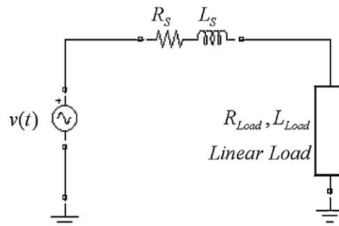
Fig. 2. Linear load supplied from a voltage source.
